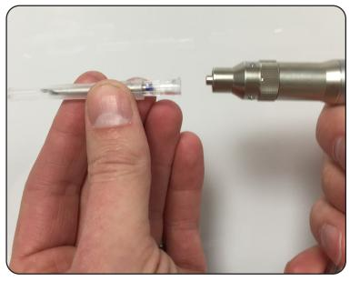
1. Insert the female luer lock transponder into the male luer lock of the transponder injector.
