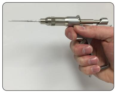
4. To set the transponder, place the needle in the animal at least 1cm and slowly squeeze the lever while maintain a fixed position. Close entry with tissue glue if needed.
