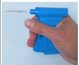
Insert the female luer lock transponder into the male luer lock of the transponder injector.
