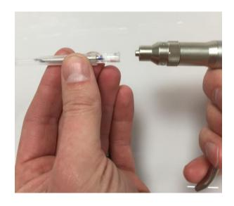
1. Insert the female luer lock transponder into the male luer lock of the transponder injector.
