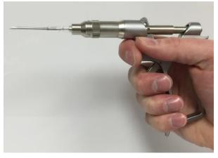
4. To set the transponder, place the needle in the animal at least 1cm and slowly squeeze the lever while maintain a fixed position. Close entry with tissue glue if needed.
