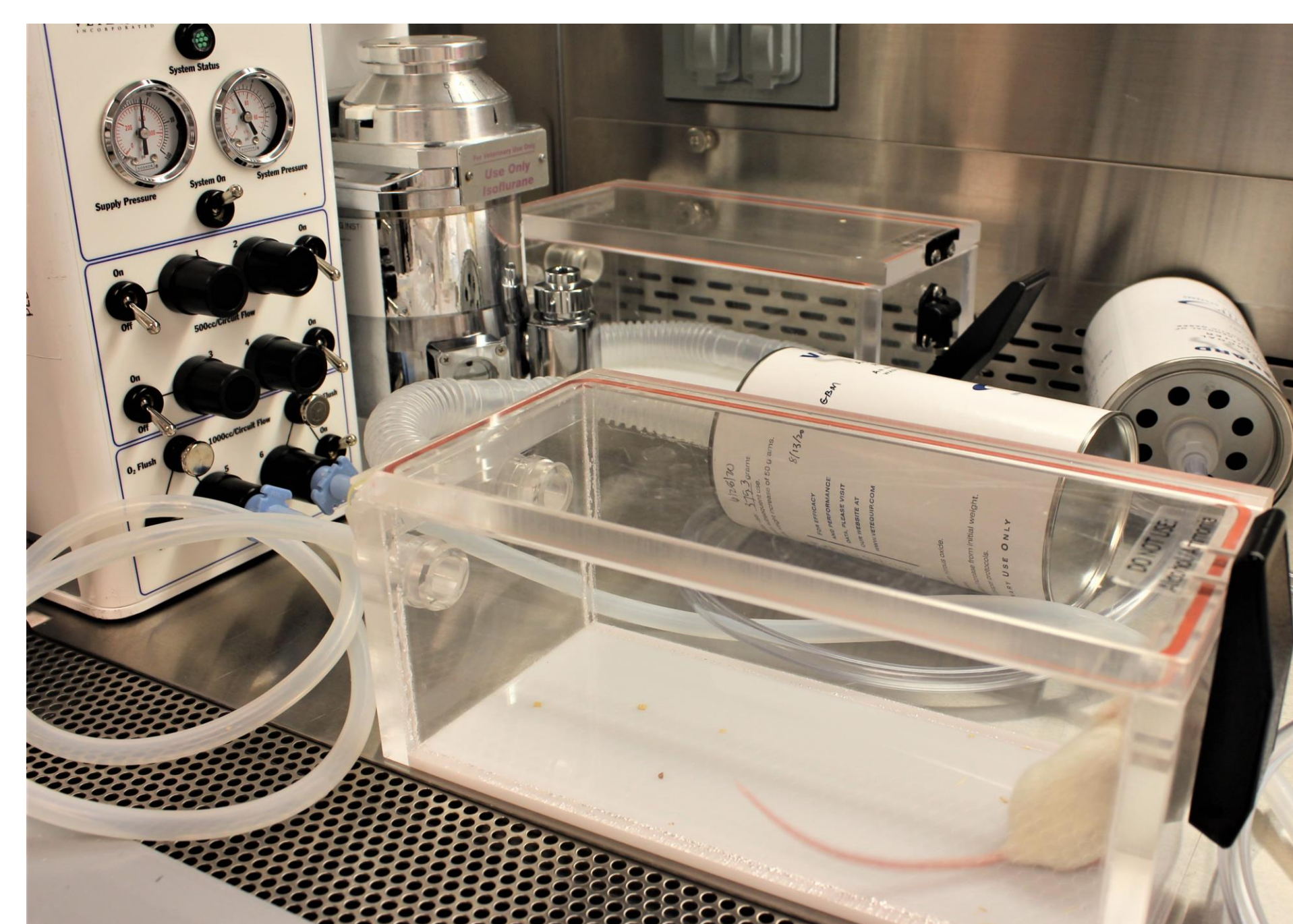
FIGURE 1. Isoflurane Chamber setup
