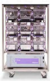
Completely compatible with modern high-density individually ventilated cage (IVC) rack systems capable of collecting spatial data for each individual animal at any given point in time.
